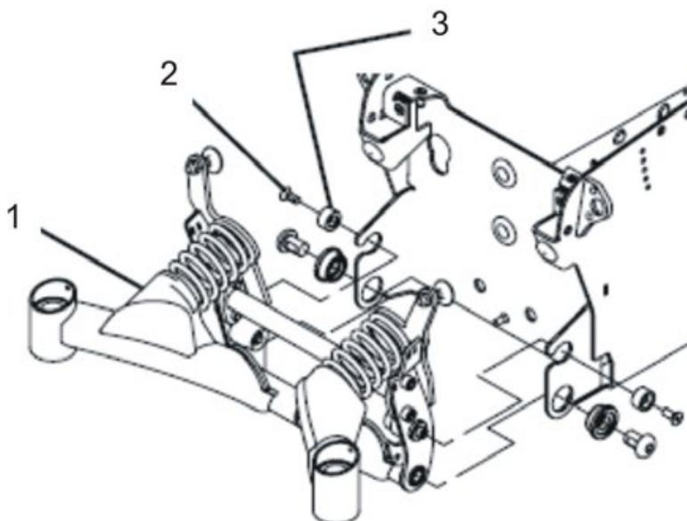
**Removing the setting screw:**
