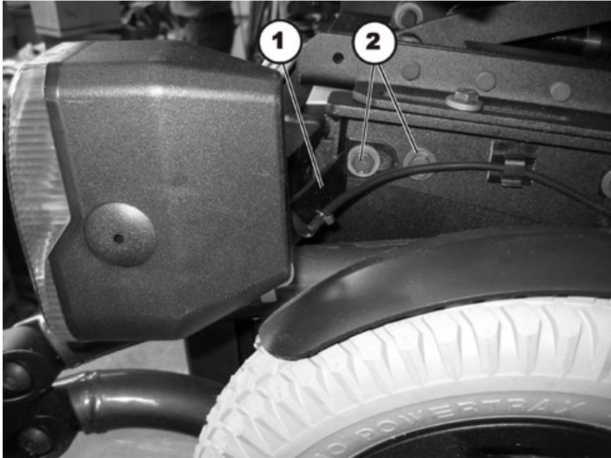
**Dismantling the bulbholder:**
