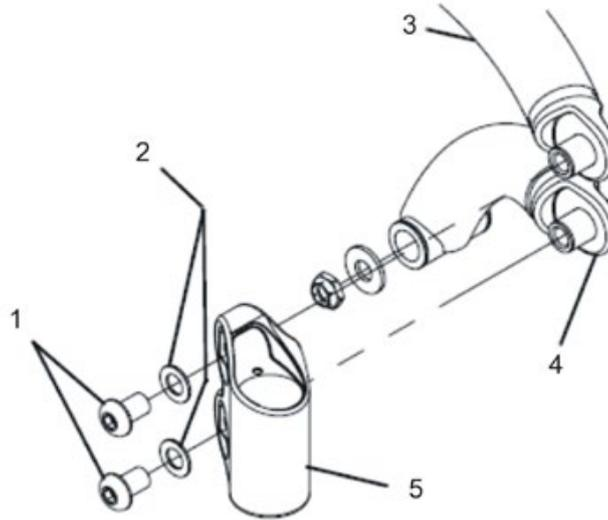
**Removing the front castor housing:**
