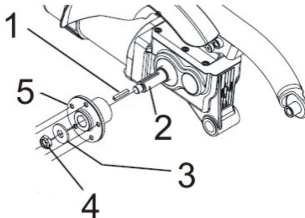
**Removing the drive wheel hub:**
