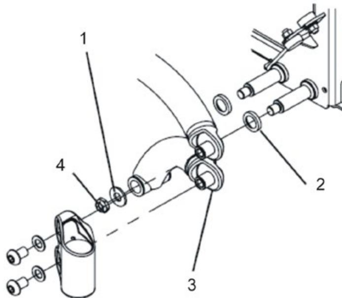
**Removing the bottom walking beam:**
