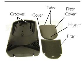
**FIGURE 2.1** Replacing the Gross Particle Filter or Filter Cover
