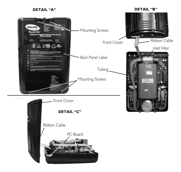
**FIGURE 2.3** Removing the Front Cover
