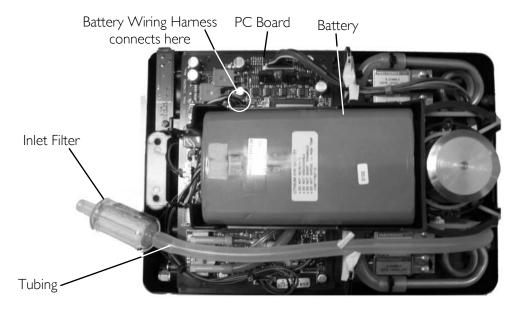
**FIGURE 2.5** Replacing the Battery
