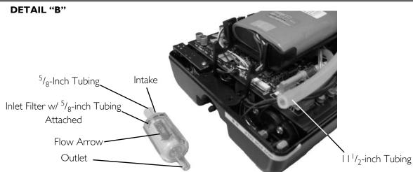
FIGURE 2.4 Replacing the Inlet Filter
