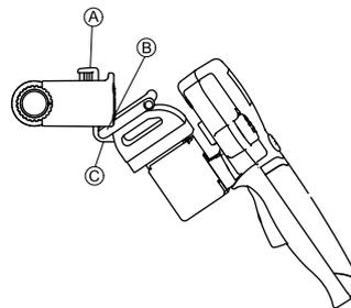
1. Remove the IDC from the adapter.
