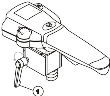
Loosen the clamping lever (1) (rotates several times!) and pull the control unit out of the wheelchair bracket.
