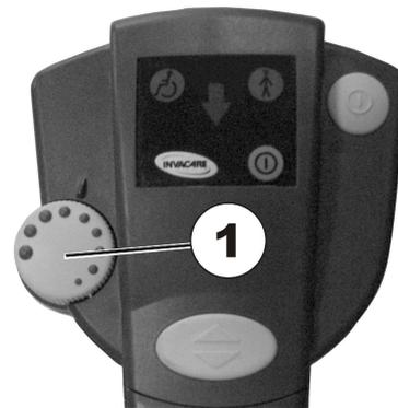
The maximum speed of the wheelchair can be set by the user to match his personal requirements and the surrounding conditions. The current maximum speed set is displayed on the wheelchair speed display and can also be preset there. You can carry out further fine adjustments to the maximum speed on the IDC using the speed potentiometer (1). In addition, the speed increases the more the drive button is pressed.
