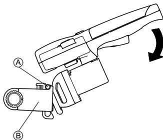
1. Position the adapter bracket (A) onto the KLIICKfix adapter (B).
