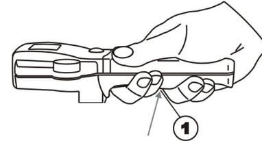
If the wheelchair needs to be stopped immediately due to a hazard situation, push the drive button (I) firmly as far as possible. This causes an immediate forced drive switch-off. Once you release the drive button (I) you can start to drive the wheelchair again immediately.
