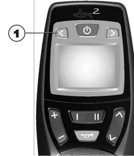
1. Press the direction indicator left key (1) for more than 3 seconds.
