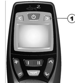
1. Press the direction indicator right key (1) for more than 3 seconds.
