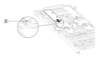
To adjust the position of the arms adjust the bolt  ${\mathfrak B}$  until the arms are in a horizontal position.
