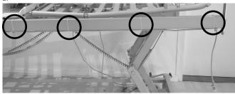
Run the motor cable underneath the bed frame toward the foot end, on both sides of the bed and fix each of the cables with zip ties onto the frame tube. Ensure that both motor cables are tighten with zip ties (marked by the circles in the picture), first zip tie near the motor and the last 3 on the frame tube toward the foot end. Make sure the end of the zip ties, are not facing outwards from the bed frame.
