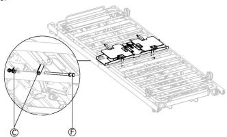
Fix the main module onto the crossbars of the mattress support frame, by placing the carrige-bolt E, trough the designated bracket on the main module C, washer and nut, from underneath on both sides of the bed.
