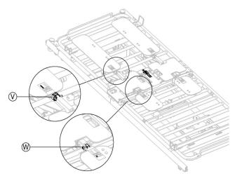
Ensure that the head arms are mounted on the telescopic bracket @ in the first threaded hole and you are not able to see the remaining threaded holes. For the foot arms make sure the telescopic bracket @, is mounted on the first threaded hole, and you are not able to see the remaining threaded holes.
