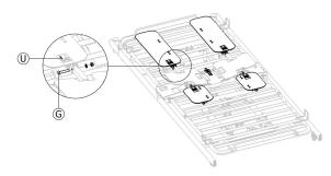
Connect the four arms with the main module, following the representation on the arms label shown in the zoomed image  $\textcircled{\tiny{0}}$ , the black shaded area on the sticker represents the location were the arm must be placed. Fix the four arms with the Allen bolts from set  $\textcircled{\tiny{6}}$  and tighten the lock nuts facing inwards. Ensure the safety washers are placed on the lock nut side.
