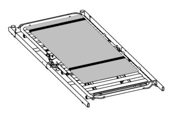
Mount the cover by sliding the pockets over the head end and foot end arms. The head end of the cover contains the label information and placement of the cover symbol:
